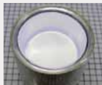
SrI 2 Packaged Scintillator
